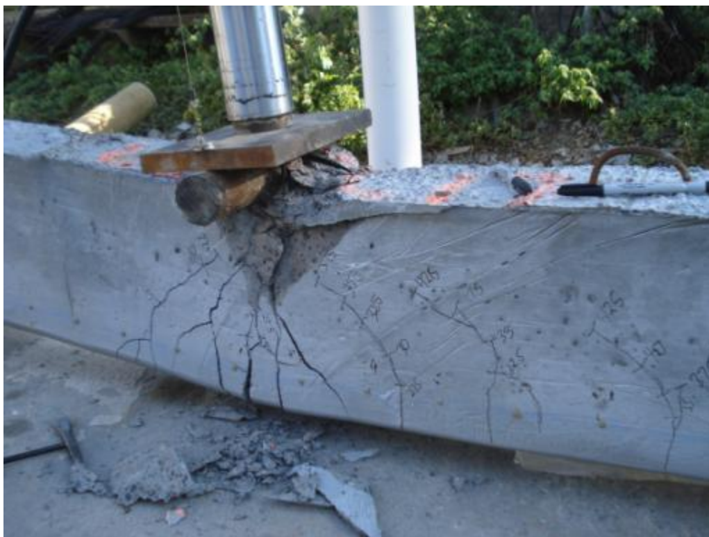
Figure 6.81: Cracking and failure of specimen HSS-4D
