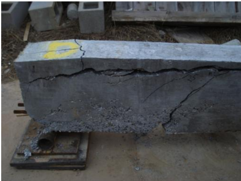
Figure 6.50: Shear cracking and failure of specimen NSL-4D
