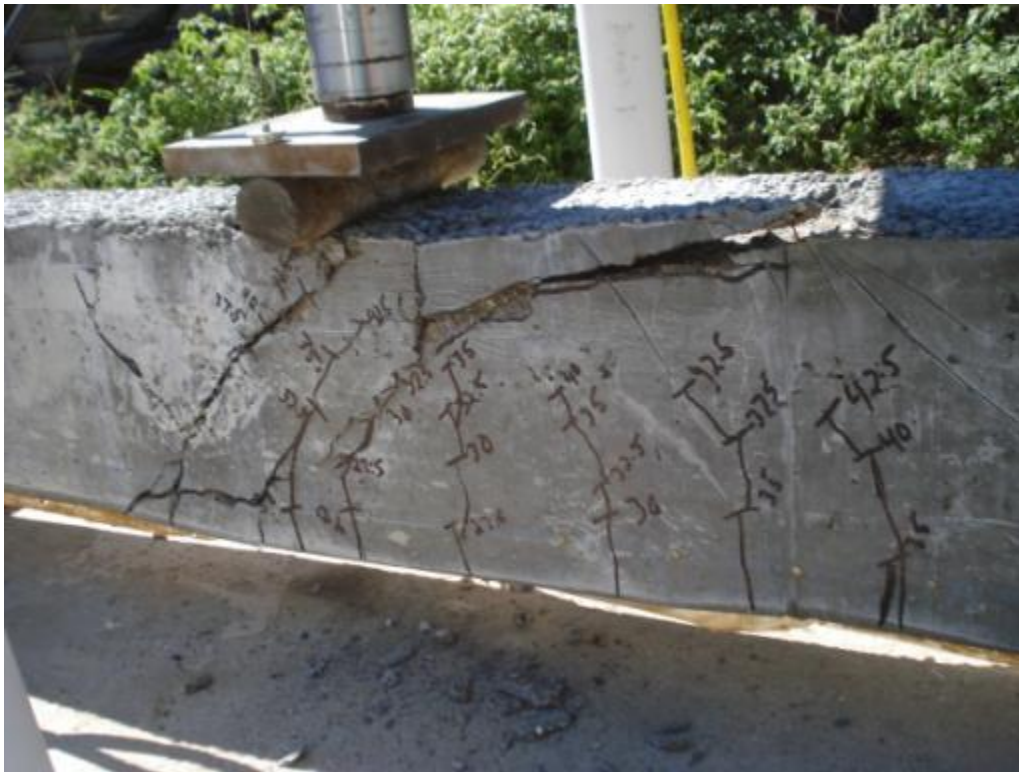
Figure 6.53: Cracking and failure of specimen HSC-1D
