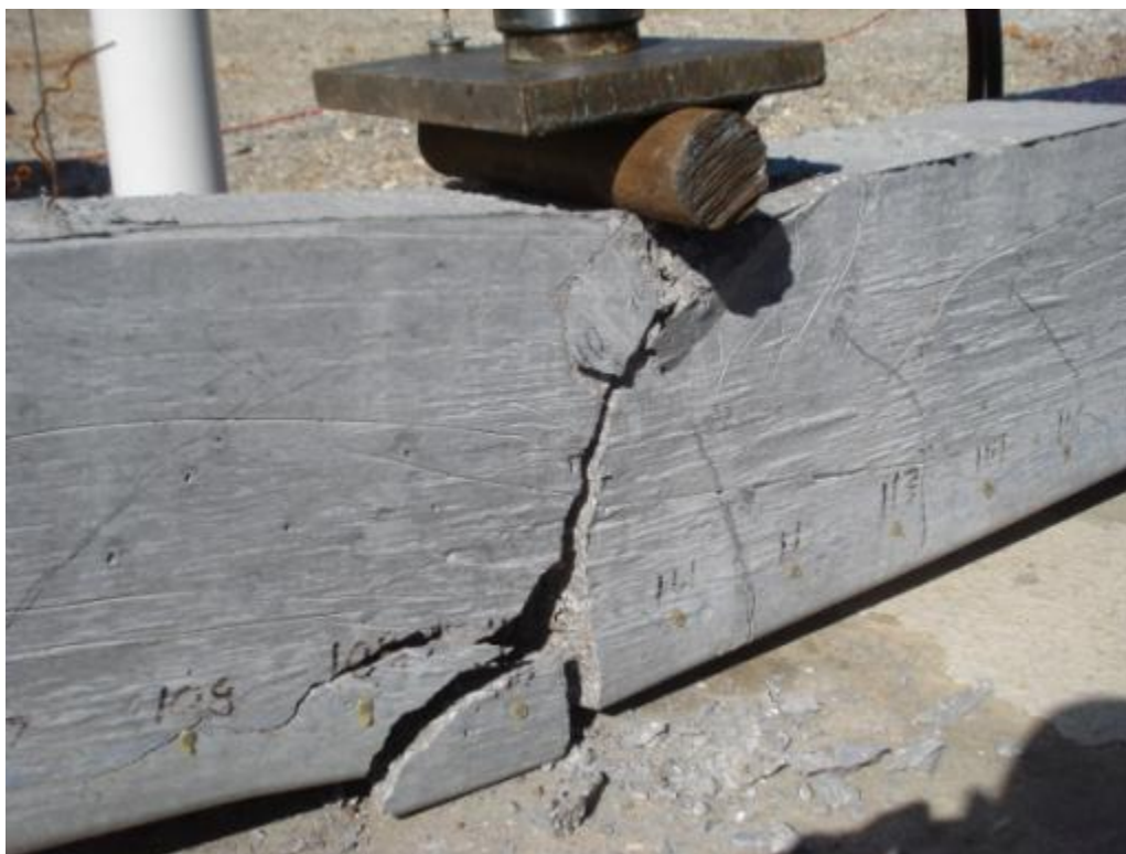
Figure 6.99: Cracking and failure of specimen HSL-4L
