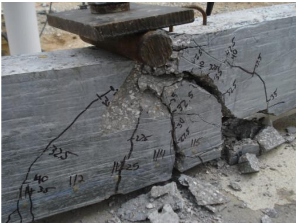
Figure 6.88: Cracking and failure of specimen HSL-1L
