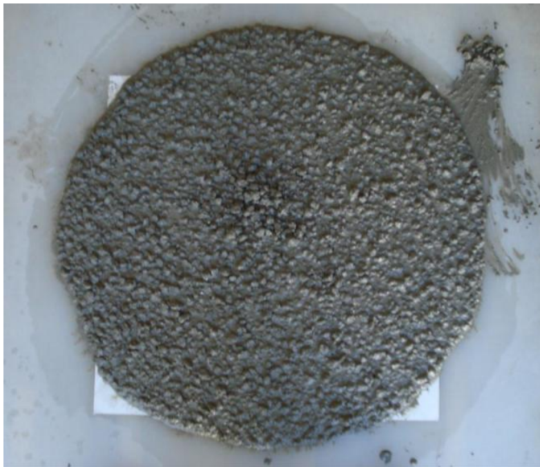
Figure 4.10: Slump flow of final HSC mixture
