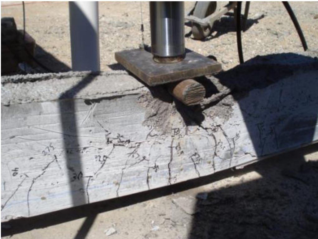
Figure 6.72: Cracking and failure of specimen HSS-1L
