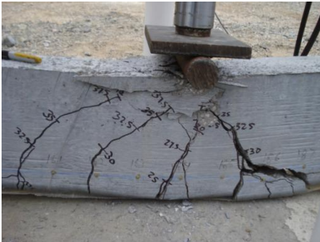
Figure 6.90: Cracking and failure of specimen HSL-2D
