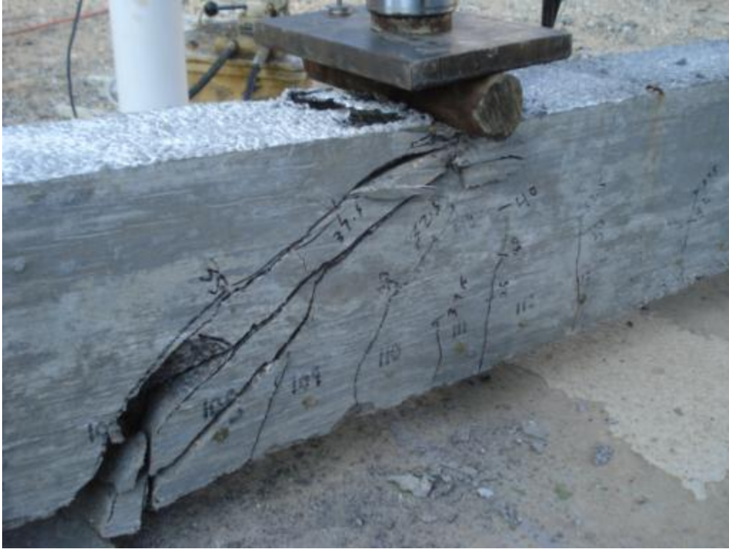
Figure 6.23: Shear failure of specimen NSS-2L
