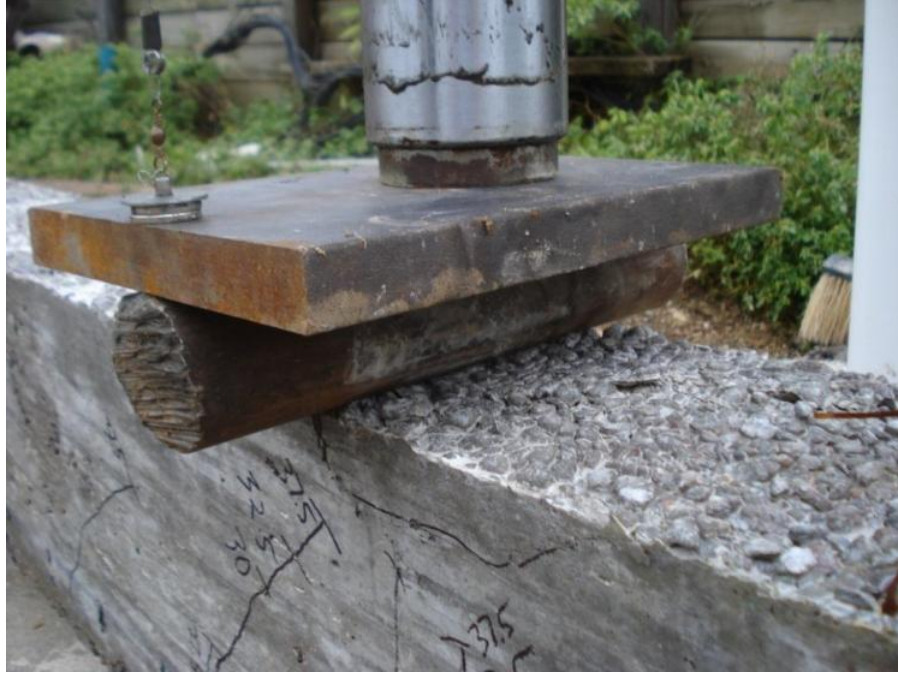
Figure 3.22: Application of point load for flexural testing
