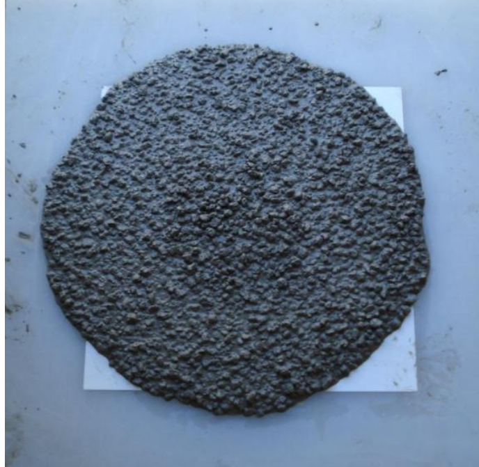
Figure 3.10: Adequate slump flow
