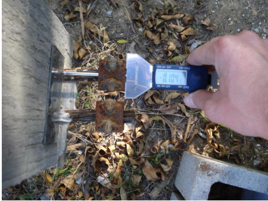
Figure 3.19: Measurement of strand end slip
