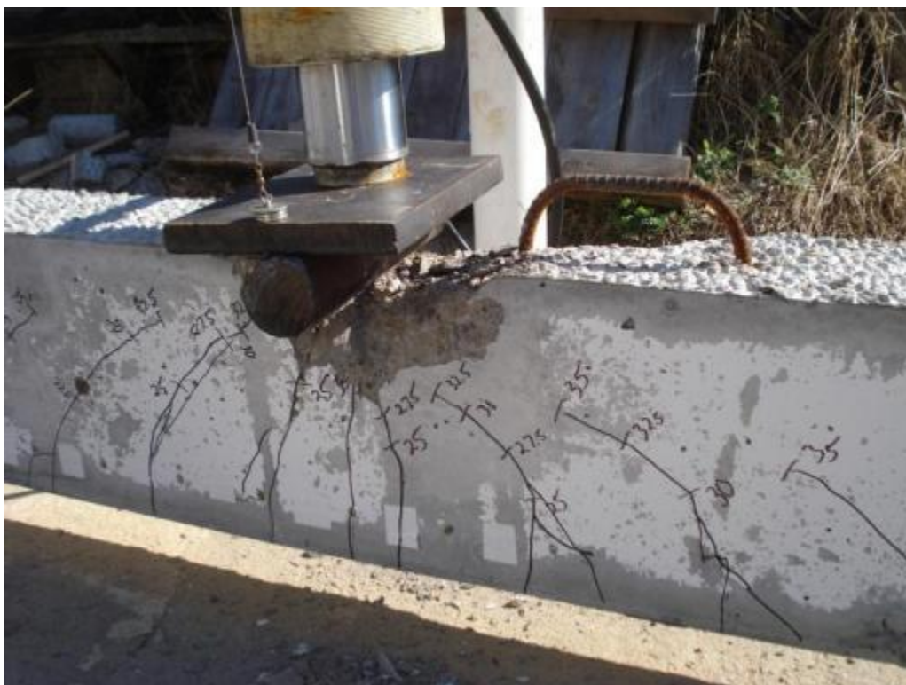
Figure 6.1: Cracking pattern of specimen NSC-1D
