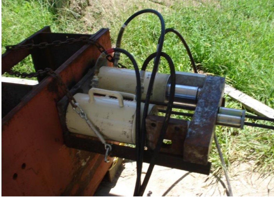
Figure 3.14: Strand tensioning apparatus with stopper blocks in place
