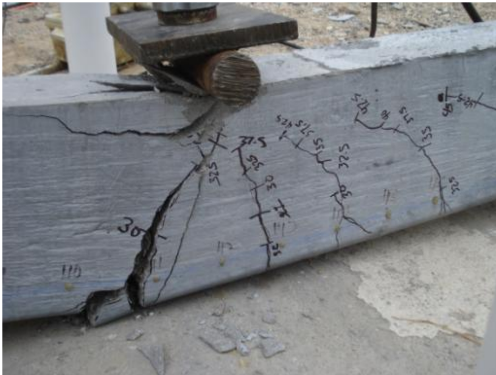
Figure 6.91: Cracking and failure of specimen HSL-2L
