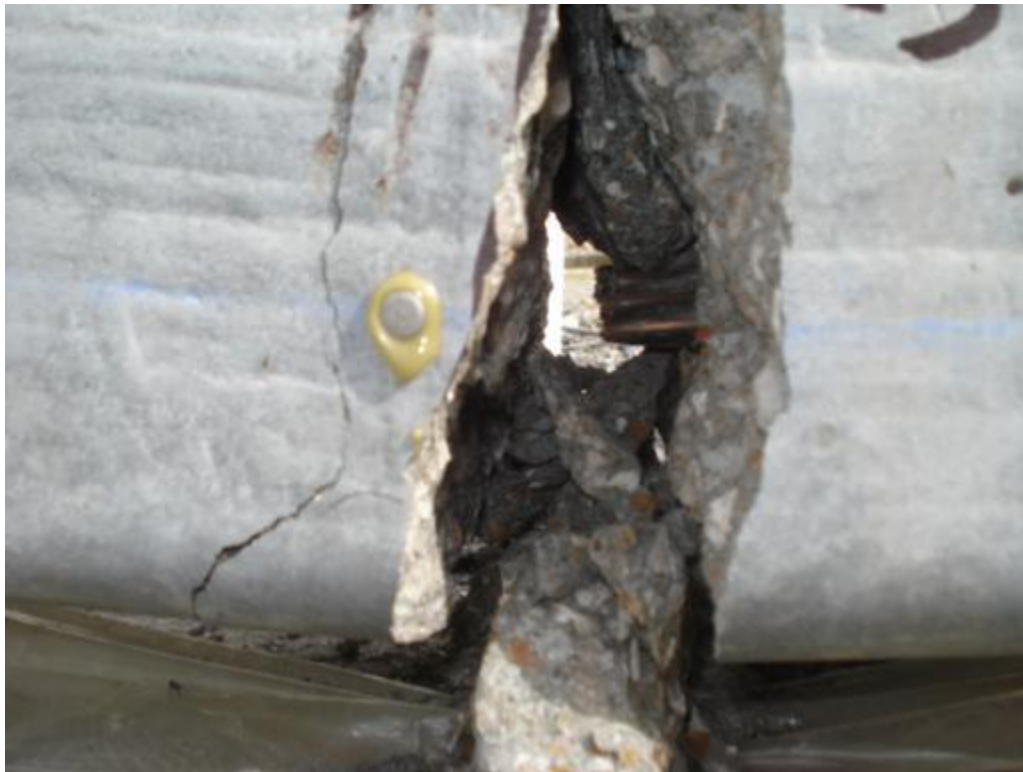
Figure 6.96: Strand fracture at failure of specimen HSL-3L
