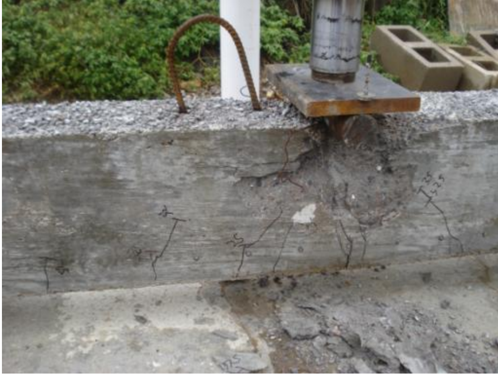
Figure 6.20: Cracking behavior and failure of specimen NSS-1L
