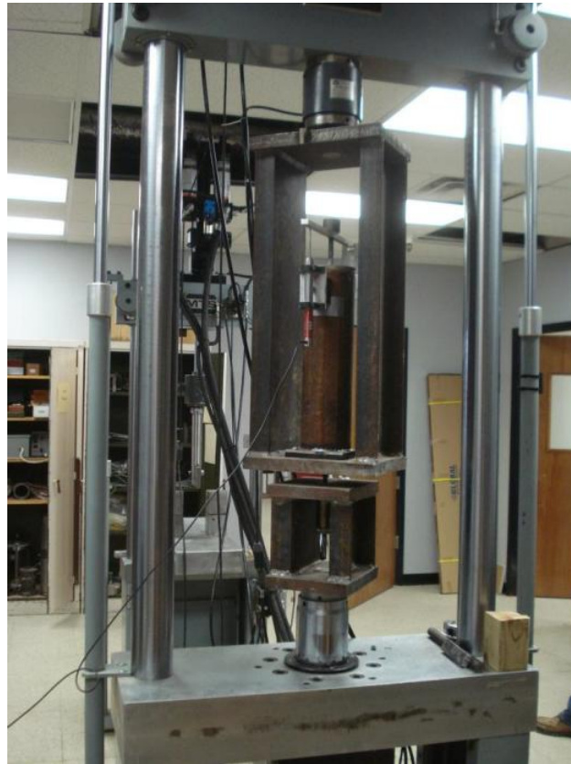
Figure 3.12: Setup for Standard Test for Strand Bond
